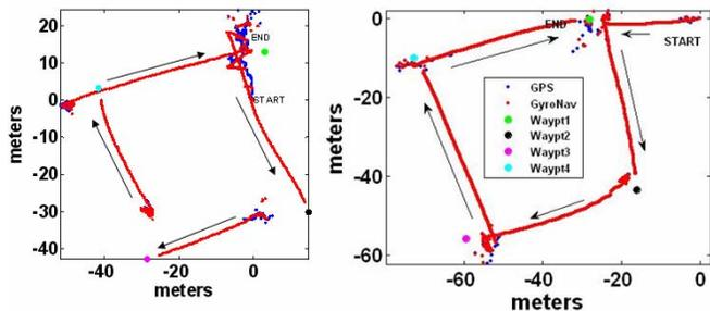
Fig. 3: Waypoint navigation. Left: using the compass heading. Right: using the gyro-integrated heading. The waypoints are shown as colored circle. GPS fixes are shown as blue dots. The vehicle's navigation is shown in red.
