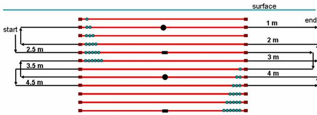
Fig. 8: Hull survey over the instrumented section of the hull
