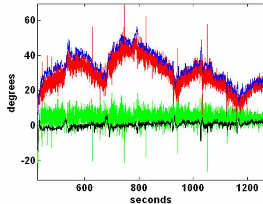
Fig. 12: Vehicle pitch (black), DVL pitch with respect to the hull (green), DVL pitch with respect to the vehicle (blue), hull inclination estimate (red).
