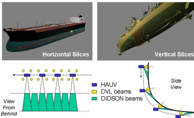
Fig. 2. Inspection by horizontal and vertical slices
