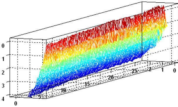
Fig. 13: 3D reconstruction of the hull section covered by the vehicle trajectory
