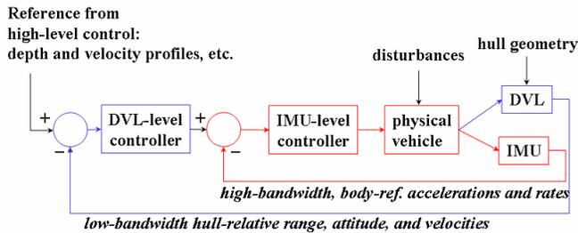
Fig. 5: Inner-outer loop control in the HAUV
