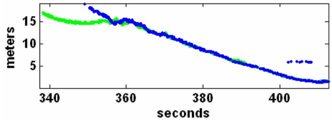
Fig. 10: Ranges reported by the two DVL beams in the horizontal plane during the "acquire" and "approach" phases
