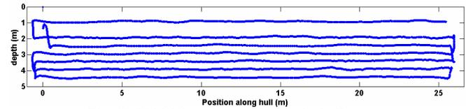
Fig. 11: Vehicle's trajectory during the hull survey
