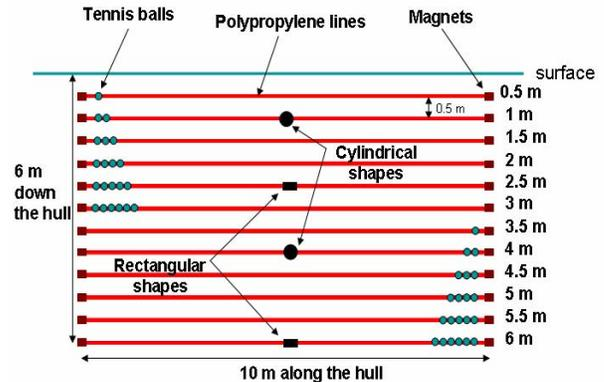
Fig. 7: Hull instrumentation to prove 100% coverage with the DIDSON
