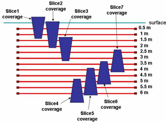
Fig. 14: DIDSON coverage for each of the slices from analysis of the DIDSON data file. Each of the trapezoidal shape slides along the lines as the vehicle executes the slice.
