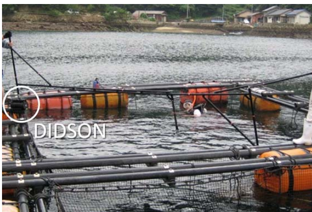
Figure 8 Showing DIDSON A installed to the pontoon by using an iron pole.
