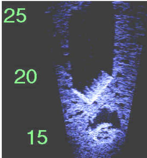
Fig. 4. A LIMIS image of a 50-gallon drum at 20 feet and an old tire at 15 feet.
