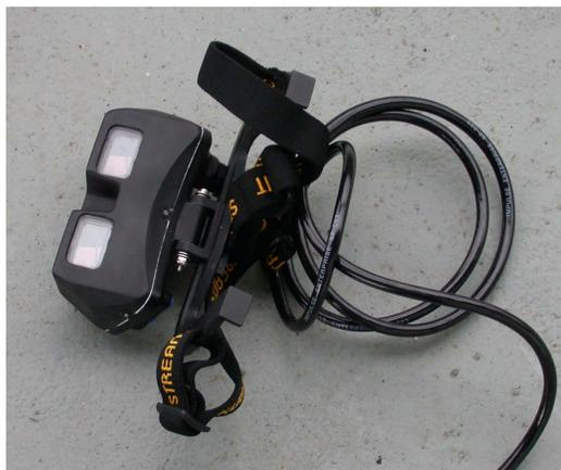
Fig. 9. Binocular version of the head-mounted display.
