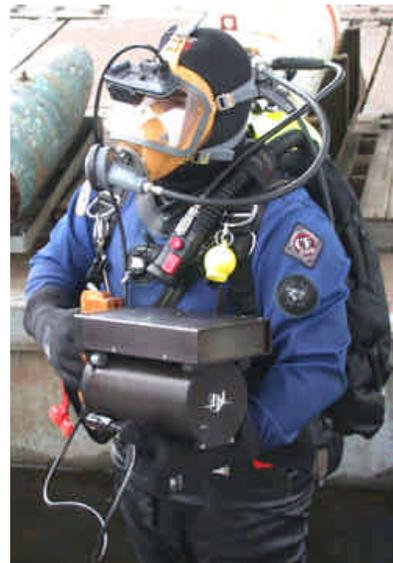
Fig. 6. A handle and head-mounted display were added to the DIDSON for this exercise. A cable connected the sonar to topside for commands and data transfer. A monocular version of the display is on the diver's mask.
