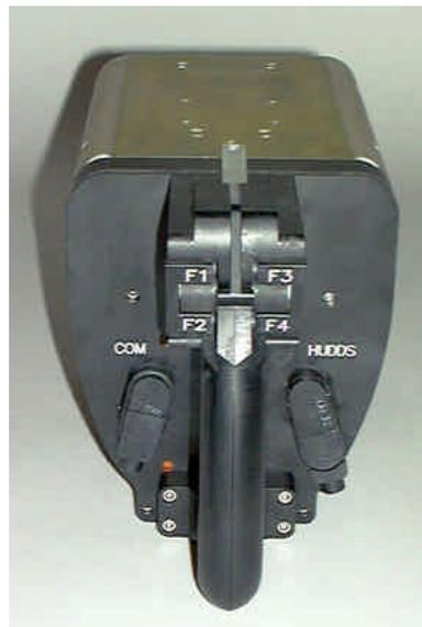
Fig. 2. Five thumb switches control the LIMIS. The four labeled F1-F4 control software commands. The fifth, between F1 and F3 controls focus. The COM port is an RS-232 link to download commands that duplicate F1-F4 controls and to upload stored digital images. The HUDDS port connects to the mask-mounted display.
