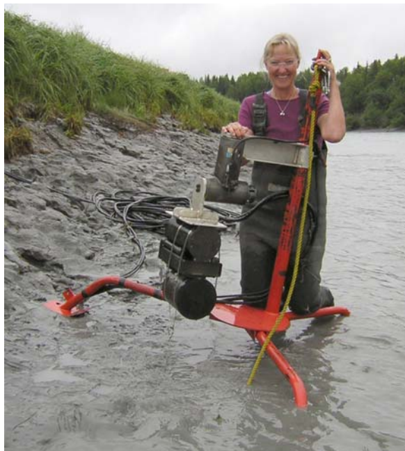
Fig. 8. Salmon are imaged with DIDSON and counted when swimming upriver to spawn in an Alaska river laden with glacial silt. (Photo courtesy of Alaska Department of Fish and Game.)
