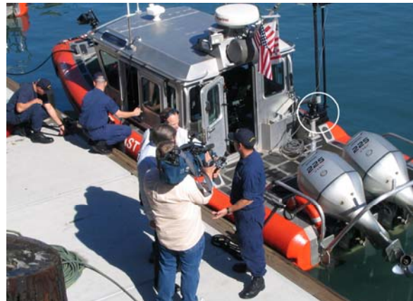
Fig. 1. U.S. Coast Guard boat with DIDSON (in circle) intercepts and verifies detected swimmer-intruders. (Courtesy of Space and Naval Warfare Systems Command.)
