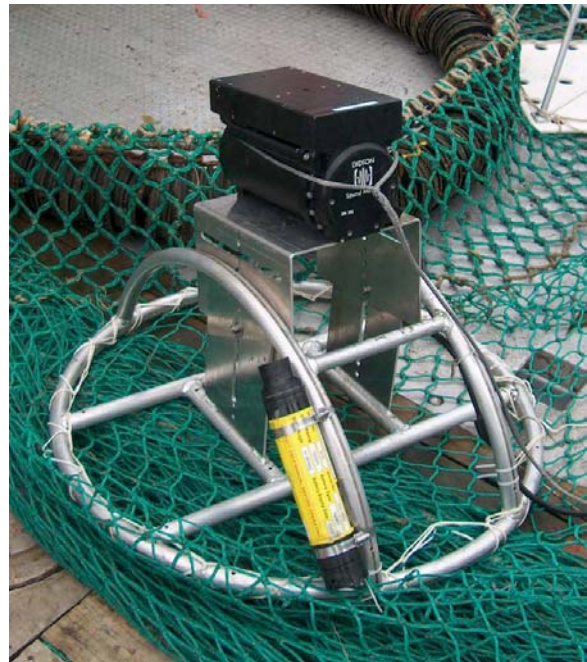
Fig. 9. The mouths of trawl nets are designed to reduce catching non-target species (bycatch). DIDSON images the fish behavior at the mouth of nets and provides needed feedback to improve the design. (Photo courtesy NOAA/NMFS/Northwest Fisheries Science Center.)
