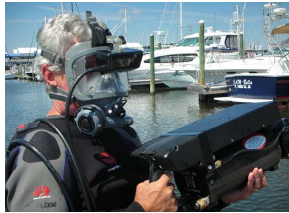
Fig. 2. Diver with mask-mounted display and diver-held model DIDSON DH. (Courtesy of Dave Elliott.)
