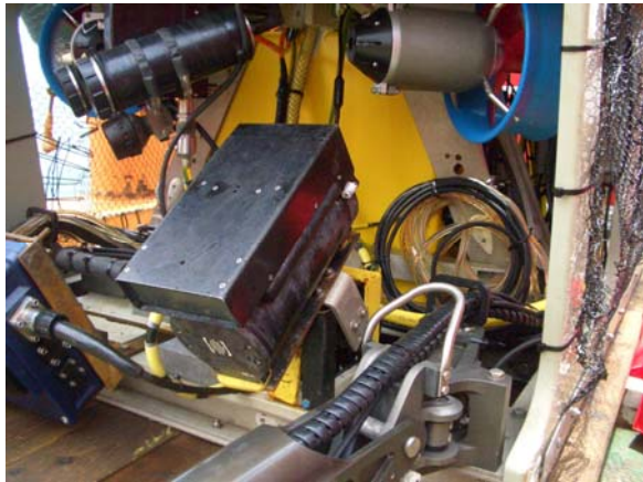
Fig. 7. The Submersible Systems, Inc. Comanche ROV uses a DIDSON for a salvage operation on a downed oil rig platform. (Courtesy of Submersible Systems, Inc.)
