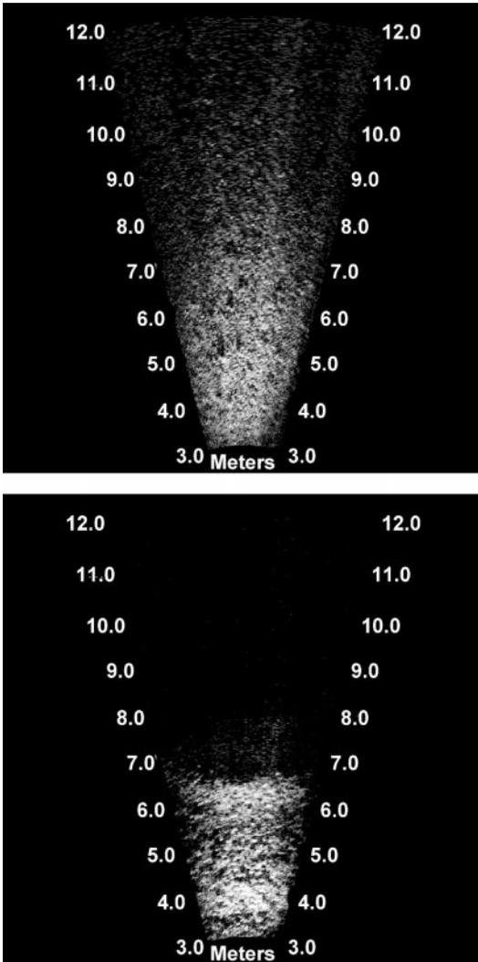
FIGURE 3.—Dual-frequency identification sonar images of an undisturbed portion of the riverbed (top panel) and a fall Chinook salmon redd (bottom panel), which appears as a dark shadow beginning at about 6.5 m.
