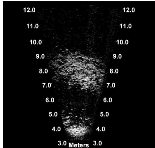
FIGURE 4.—A dual-frequency identification sonar image showing two fall Chinook salmon redds, one beginning at about 4.5 m and the other at 9.0 m.
