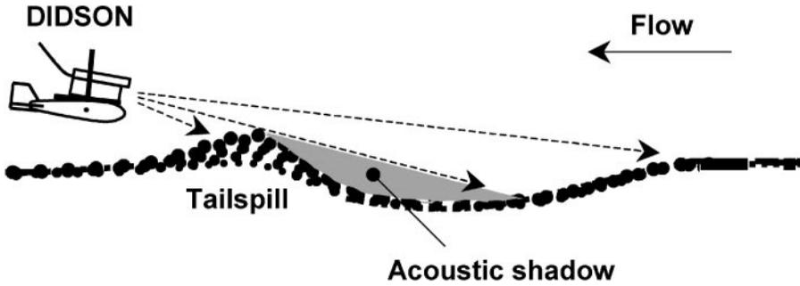
FIGURE 1.—A conceptual depiction of the way in which the morphology of a fall Chinook salmon redd enables acoustic imaging by a dual-frequency identification sonar (DIDSON).
