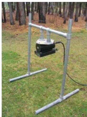
Figure 1 – Illustration of the DIDSON-LR mounted on the stand.
