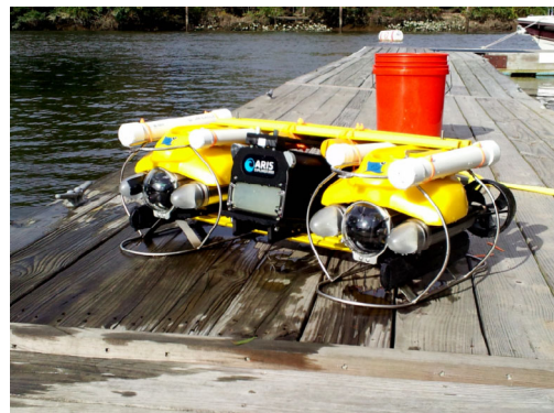
Captured: ARIS Explorer 3000 mounted to two ROVs
