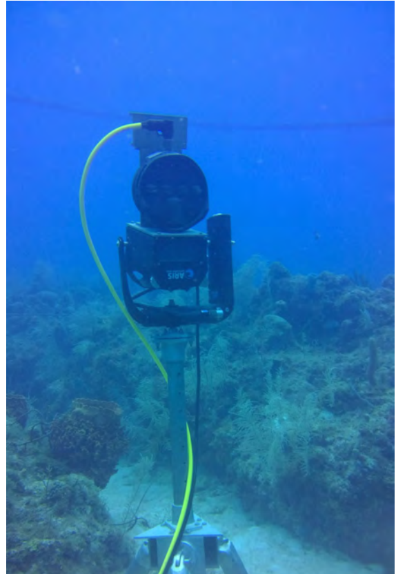
Pictured above: An outside view of Aquarius, and the ARIS Explorer 3000 employed on the ocean floor
