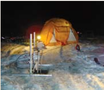
DIDSON set up to check the short lamprey run on the Yukon River
